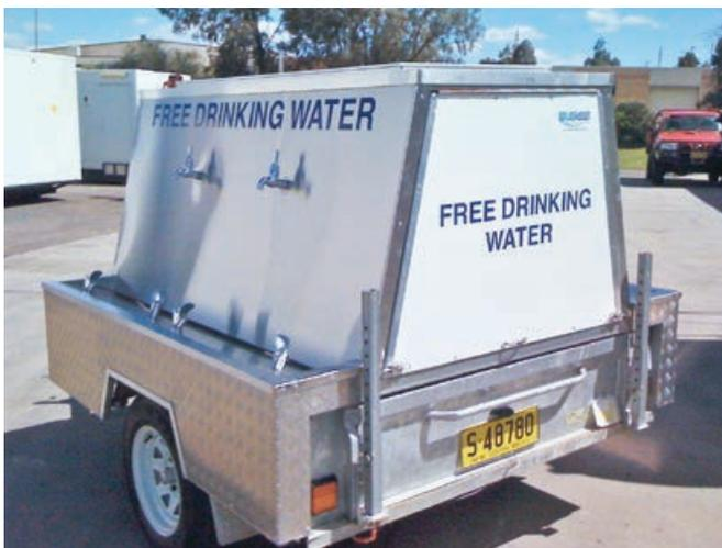
Option 3: 8 bubbler and 4 tap hydration trailer with 600 L holding tank. Can also connect to mains water.
